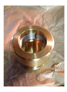
5) Insert pipe beyond the o-ring and tighten by hand. **HAND TIGHT WILL BE SUFFICIENT**
