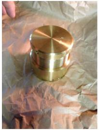
4) Invert assembly (Be sure the INSERTS do not fall out of the NUT) and insert the pipe into the ENDCAP. You will feel the resistance of the o-ring.
