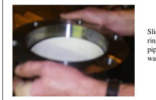
Slide top assembly ring housing on pipe. Slide it all the way down the pipe.
