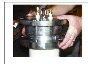
Slide clamp ring housing up over the inserts and bolt on. Follow same bolt procedure as the bottom assembly.
