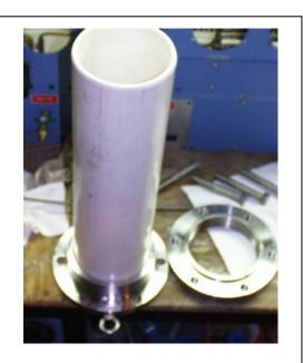
Inserting pipe into bottom endcap assembly
